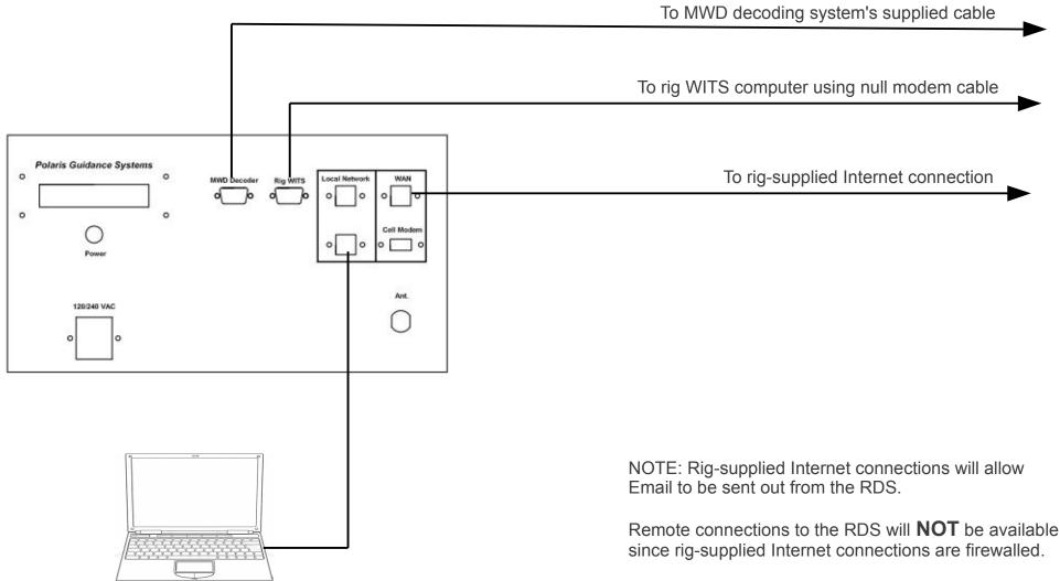
Laptop Ethernet adapter settings should be DHCP or automatic. Wireless should be disabled so it doesn't interfere with Ethernet communications.
