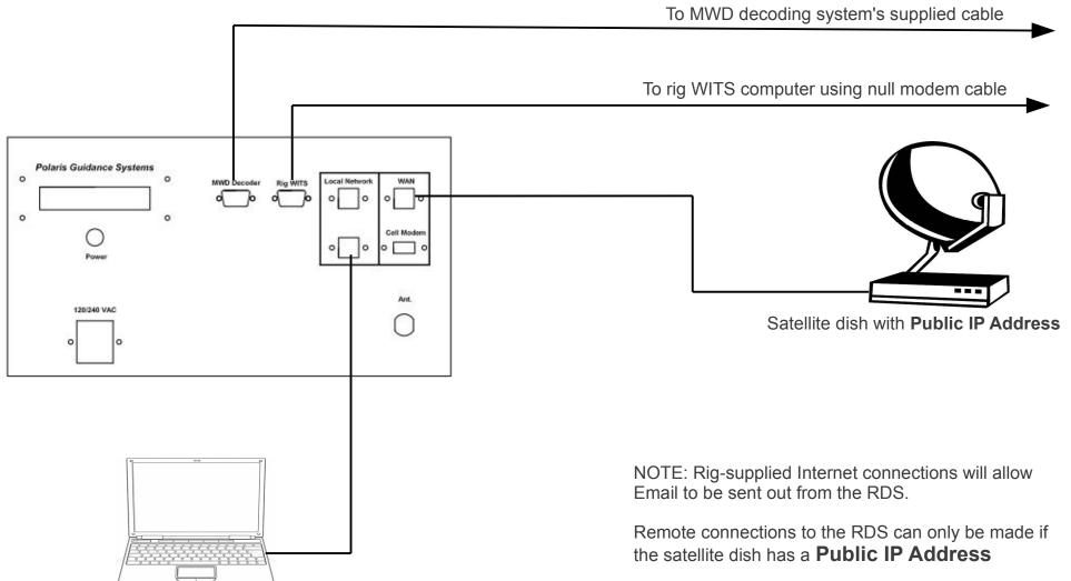
Laptop Ethernet adapter settings should be DHCP or automatic. Wireless should be disabled so it doesn't interfere with Ethernet communications. Please contact your satellite provider and ask for a Public IP Address
