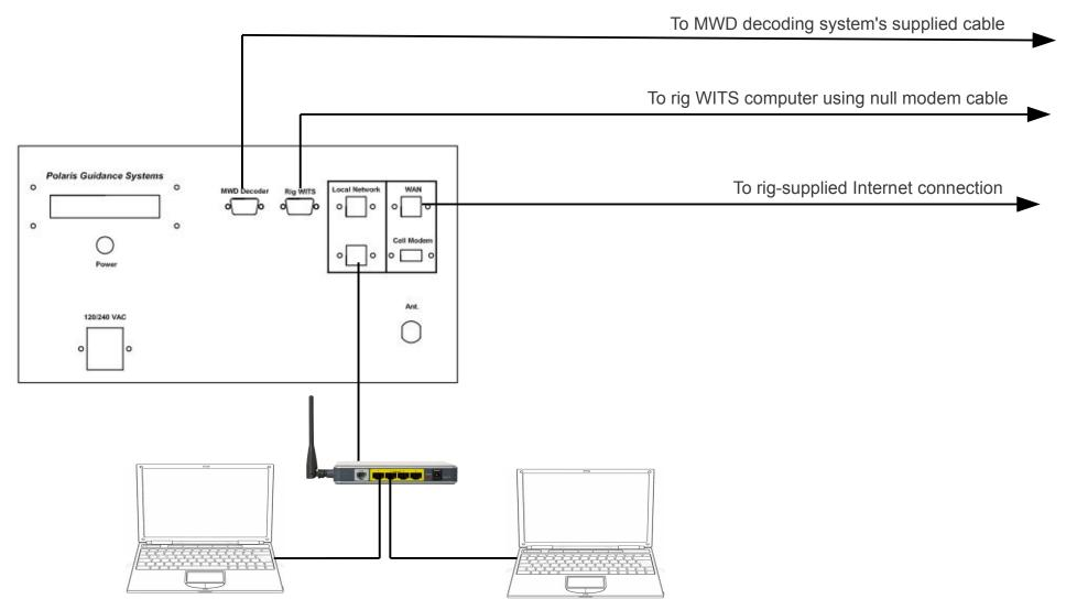
Laptop Ethernet adapter settings should be DHCP or automatic. Wireless should be disabled so it doesn't interfere with Ethernet communications.
